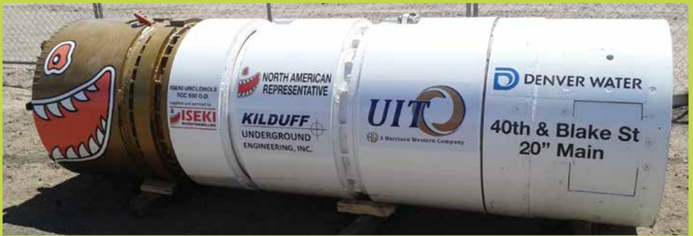
The Iseki Unclemole used for the 410-ft crossing for Denver Water.
